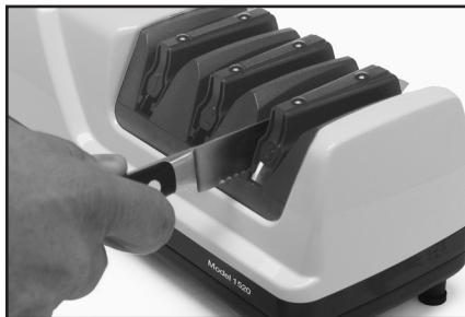
Figure 14. Use only Stage 3 for sharpening serrated knives.
